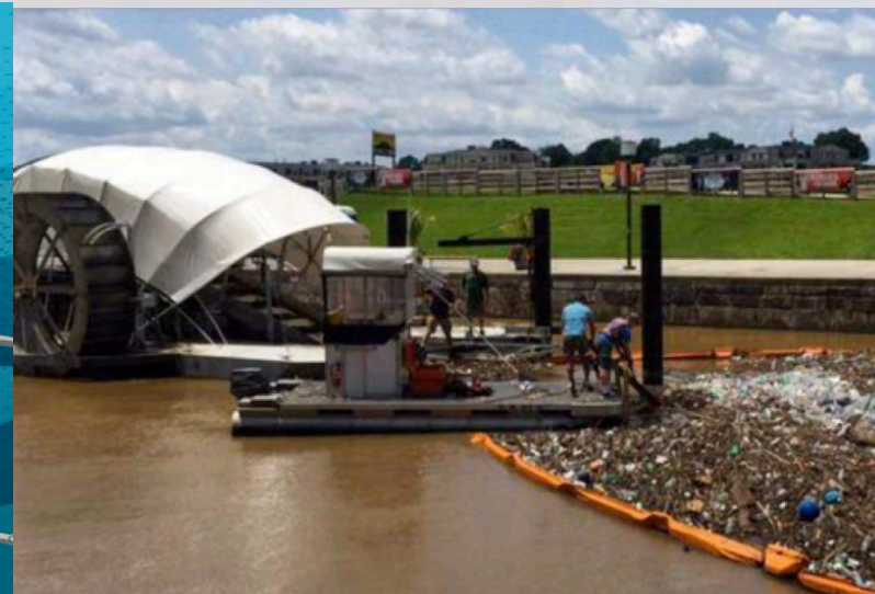
Trash Wheel - A hydro-solar powered water wheel captures trash in international waters, a solution to pollution.
